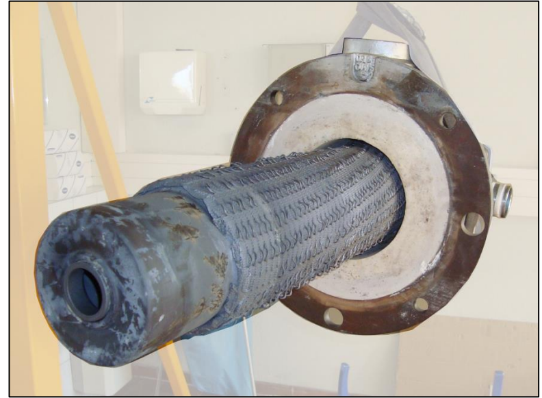
heat exchanger with Geometry 1
