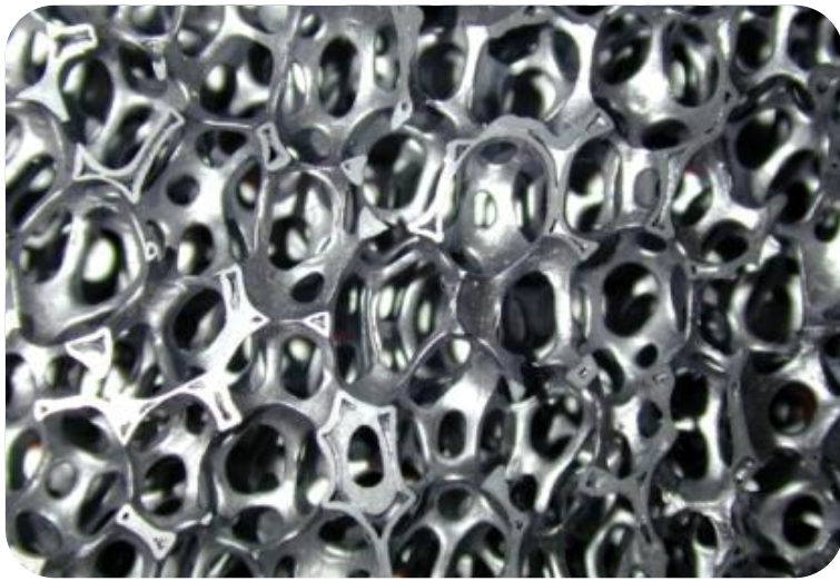
SiSiC foam, Erbicol SA, 3-dimensional flow
